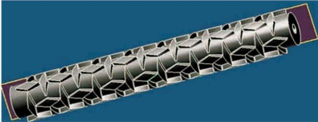
**Figure 5: A 3D design of Auxetic (reverse) tubular die**
