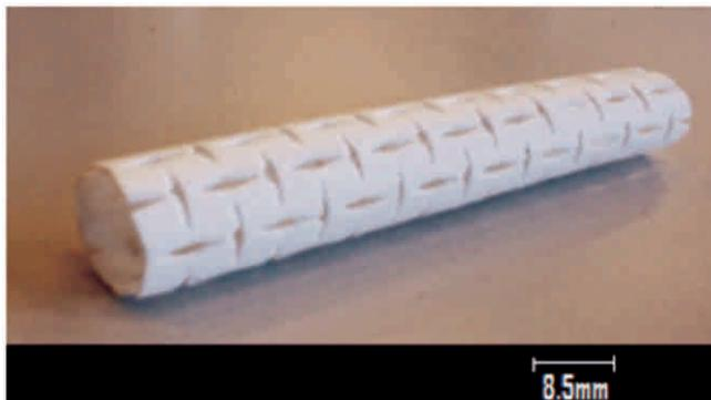
**Figure 13: Auxetic airway stent developed seamlessly by using polyurethane material**
