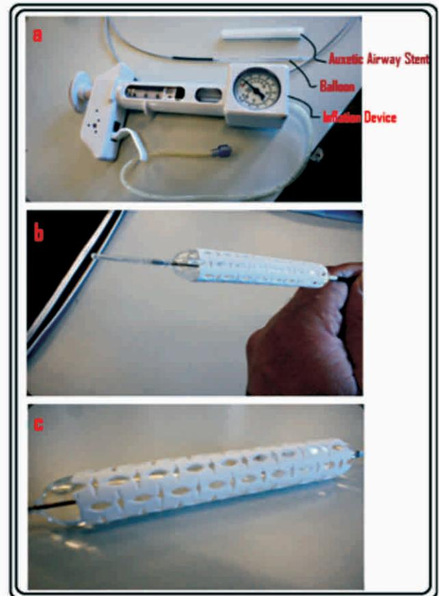
**Figure 14: (a) Auxetic airway stent along with balloon catheter and inflation device, (b) Auxetic stent mounted on a balloon catheter and (c) axial length and diameter of the stent is being checked at different pressures**
