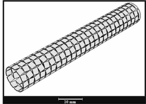
Figure 3: Schematic showing an Auxetic airway stent
