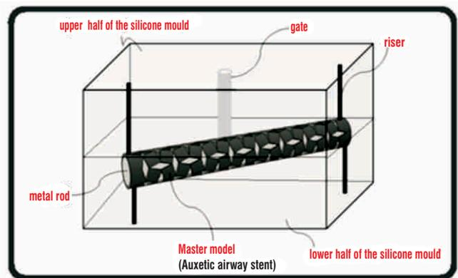
**Figure 12:** A schematic showing Master model suspended inside the silicone mould
