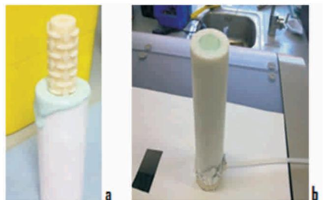
**Figure 8: (a) Reverse-Auxetic template being pushed inside a TEFLON tube, and (b) silicone elastomer casted onto an antipode-Auxetic template inside the TEFLON tube**
