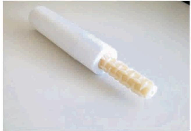
**Figure 7: A tubular template is fixed tightly within TEFLON tube**
