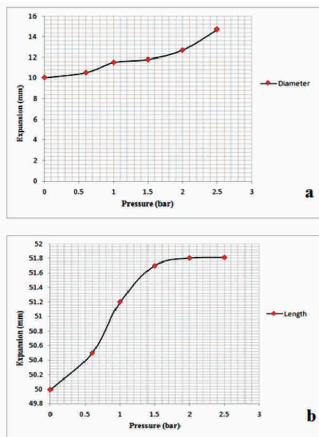
**Figure 15: (a) A graph showing diametrical changes of an Auxetic airway stent, and (b) a graph showing the longitudinal extension of the stent**
