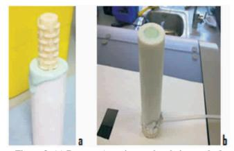
Figure 8: (a) Reverse-Auxetic template being pushed inside a TEFLON tube, and (b)silicone elastomer casted onto an antipode-Auxetic template inside the TEFLON tube
