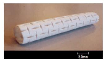
Figure 13:Auxetic airway stent developed seamlessly by using polyurethane material
