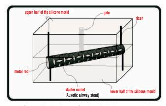
Figure 12: A schematic showing Master model suspended inside the silicone mould
