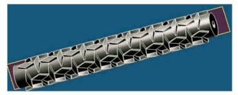
Figure 5: A3D design of Auxetic (reverse) tubular die
