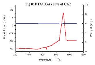
First endothermic peak in this case is observed at 660 °C which corresponds to the melting of aluminum metal as shown in Figure 8. This peak is followed by a sharp exothermic peak at 890 °C which is the ignition temperature of the composition under these conditions. The use of Si +  $Bi_2O_3$  (mass ratio 1:4) as sensitizer for the Al+ CuO plus thermite reaction, lowers the ignition temperature of the system from 1020 to 890 °C.
