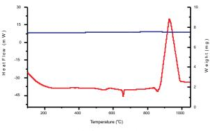
Fig 6: DTA/TGA curve of PbA1
