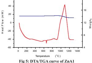
First endothermic peak is observed at  $660 \,^{\circ}\text{C}$  shown in Figure 5 which indicates the melting of aluminum. Then at
