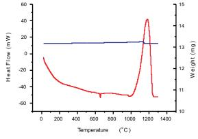
Fig 3: DTA/TGA curve of nFeA3
