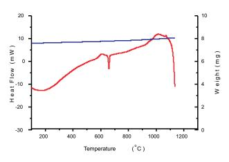
Fig 1: DTA/TGA curve of FeA1
