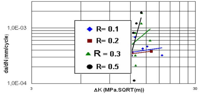
**Fig. 4. Striation spacing at different load ratio [23]**
