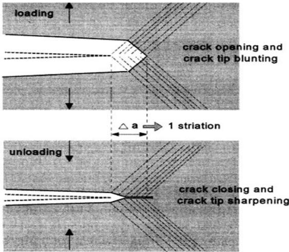
**Fig. 2. Crack tip blunting and re-sharpening mechanism [17]**
