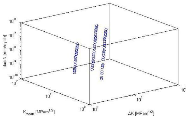
**Fig. 11. Crack growth data  $\frac{da}{dN}$  verses  $\Delta K$  and  $K_{mean}$  [30]**
