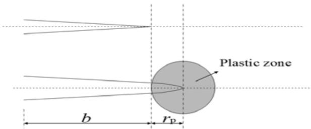
**Fig. 6.** Plastic zone size formation mechanism [11]
