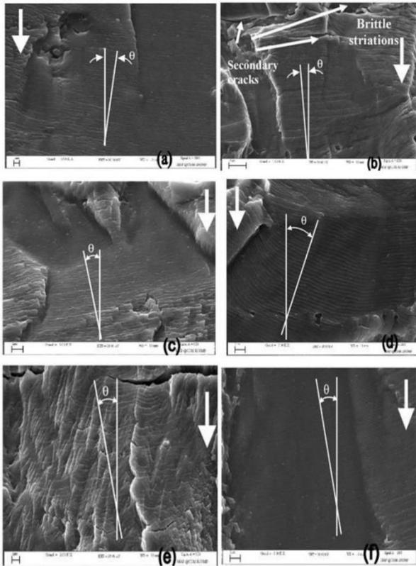
**Fig. 3. Fatigue striation spacing at different load ratio [23]**
