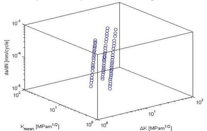
**Fig. 8.** Crack growth data  $\frac{da}{dN}$  versus  $\Delta K$  and  $K_{\text{mean}}$  [29]
