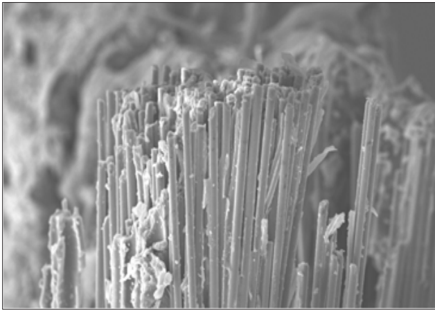
Fig.2: SEM image of carbon fiber epoxy composite
