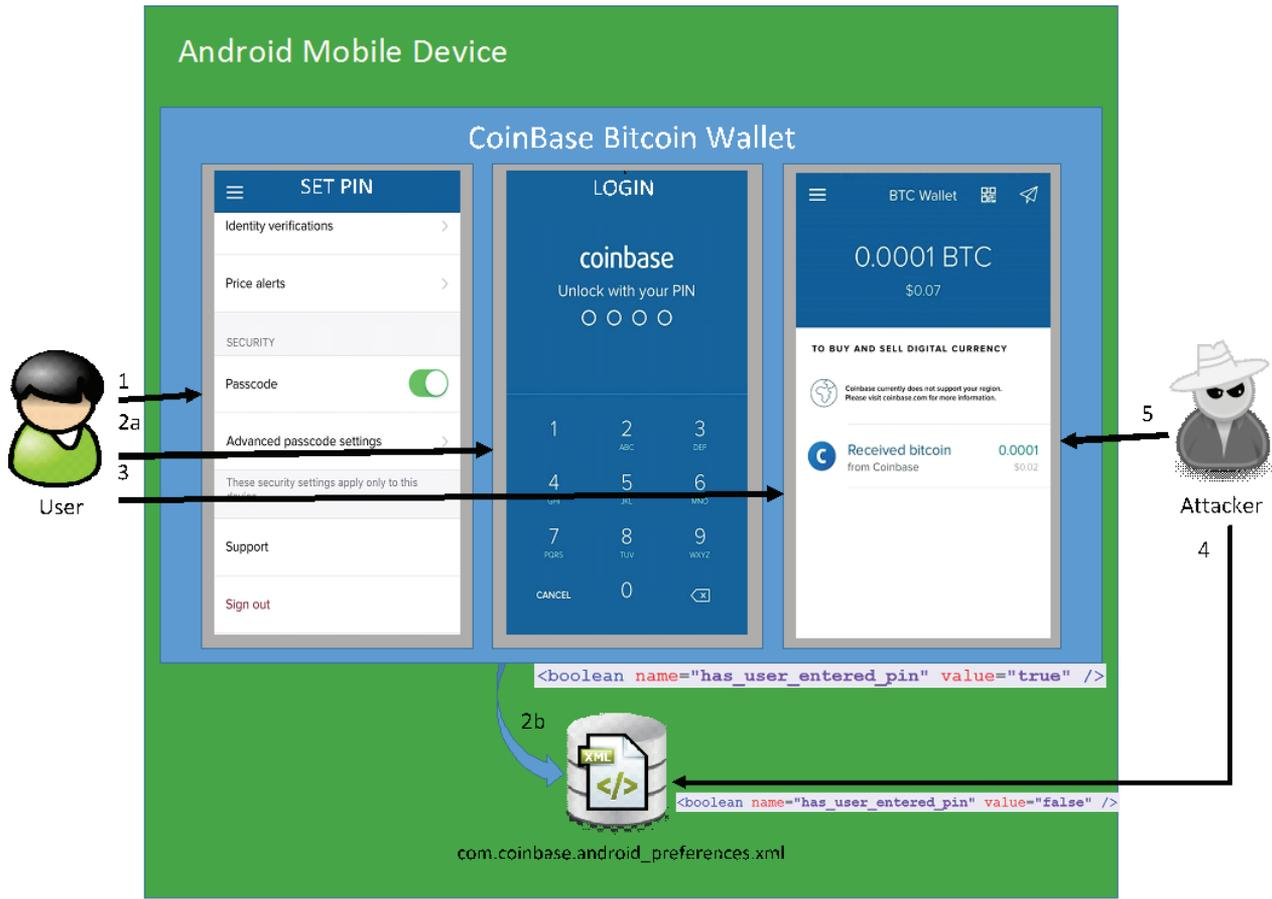
Figure 1 Coinbase Bitcoin Wallet Authentication Bypass
