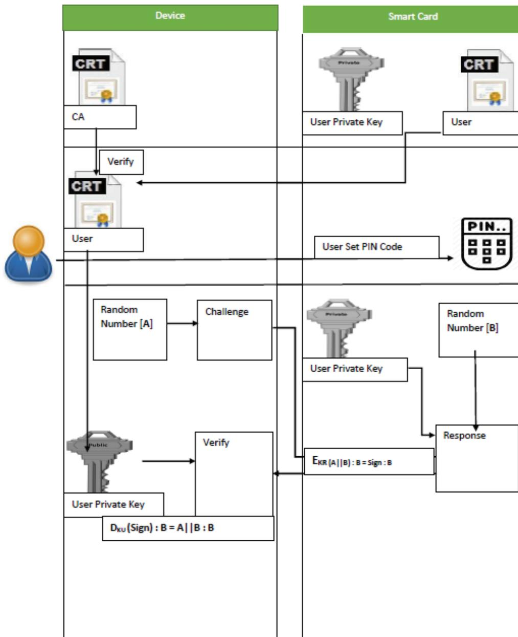
Fig. 4: Smart Card based Authentication
