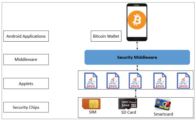
Figure 3 Smart Card based Bitcoin Application's Architecture
