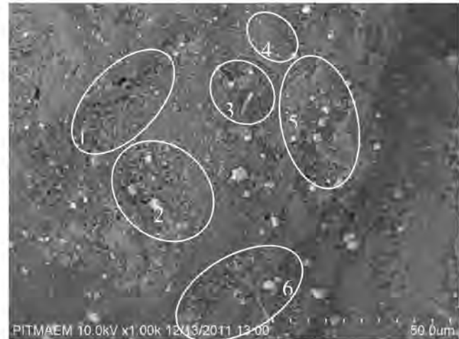
(h) Sand sample taken after casting (SEM image at mag. x1000) particles of phosphoric acid and cementitious compounds (1-6)
