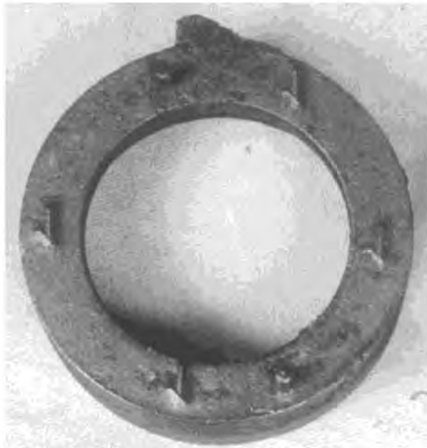
(a) Moulding sand + tartaric acid 2% (good surface finish )
