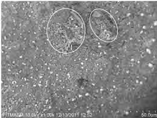
(g) Sand sample taken after casting (SEM image at mag. x1000 particles of phosphoric acid sticking with grains, and cementitious compounds (1,2)
