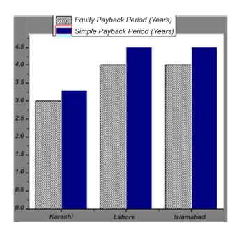
Fig 5: Equity and simple payback periods of stand-alone PV system
