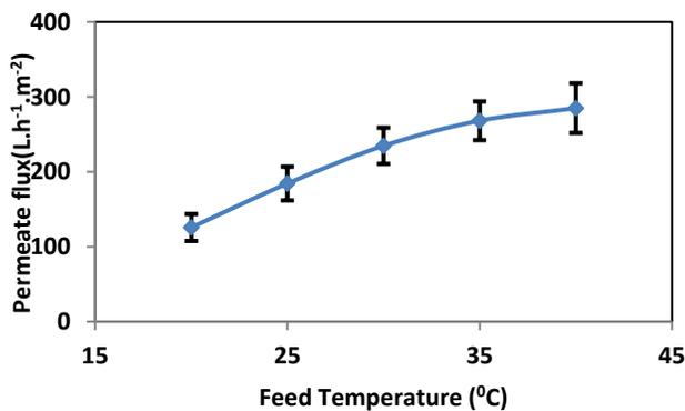
**Fig. 3: Effect of feed temperature on permeate flux (mean ± SD). Feed flow rate and TMP 3 Bar in Total recycle mode were kept constant at 11 L.min<sup>-1</sup> and 3 bar respectively (n=3 for each feed temperature).**
