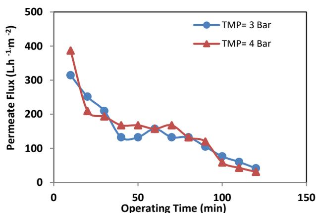
**Fig. 6:** Effect of operating time on permeate flux of apple juice (Feed flow rate: 11 L.h<sup>-1</sup>.m<sup>-2</sup>), Concentration mode.
