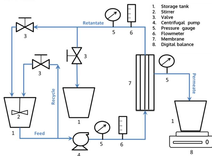
**Fig. 1: Laboratory scale Crossflow microfiltration unit.**
