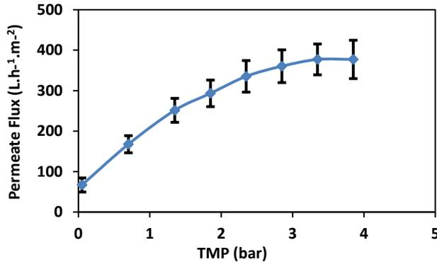
**Fig. 2: Influence of TMP on permeate flux (mean ± SD). Feed flow rate and temperature in Total recycle mode were kept constant at 20°C and 11 L.min<sup>-1</sup> respectively (n=3 for each TMP).**
