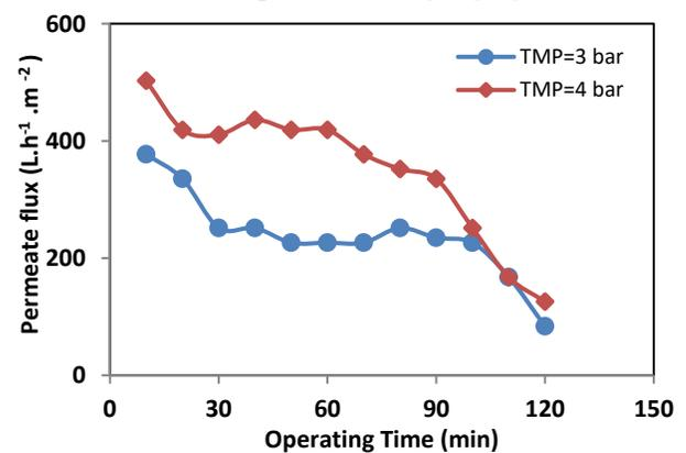
**Fig. 5: Effect of operating time on Permeate flux at different TMP (Feed flow rate: 11 L.h<sup>-1</sup>.m<sup>-2</sup>), Total recycle mode.**
