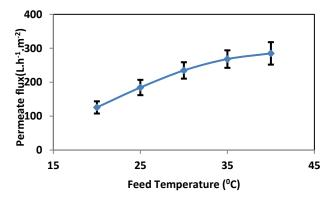
Fig. 3: Effect of feed temperature on permeate flux (mean  $\pm$  SD). Feed flow rate and TMP 3 Bar in Total recycle mode were kept constant at 11 L.min<sup>-1</sup> and 3 bar respectively (n=3 for each feed temperature).
