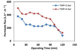
Fig. 5: Effect of operating time on Permeate flux at different TMP (Feed flow rate: 11 L.h<sup>-1</sup>.m<sup>-2</sup>), Total recycle mode.
