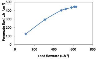
Fig. 4: Effect of Feed flowrate on Permeate flux (Temperature: 20 °C, TMP: 3 Bar) Total recycle mode.
