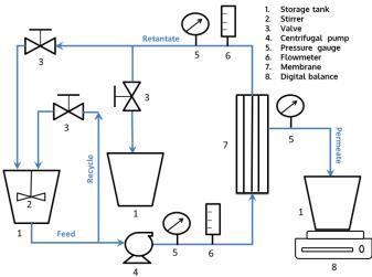
Fig. 1: Laboratory scale Crossflow microfiltration unit.
