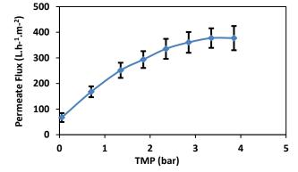
Fig. 2: Influence of TMP on permeate flux (mean  $\pm$  SD). Feed flow rate and temperature in Total recycle mode were kept constant at 20<sup>o</sup>C and 11 L.min<sup>-1</sup> respectively (n=3 for each TMP).
