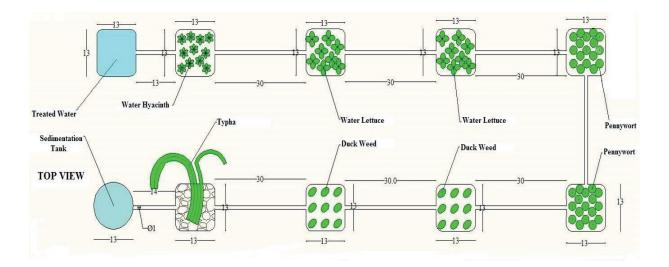
Fig-1: Layout of Lab Scale and Pilot Scale Treatment System
