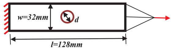
Fig-4: Dimensions of base line specimen
